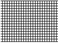
Guardian features black powder coated 304 stainless steel mesh. The 0.6mm diameter wire has a 1.3mm aperture providing an open area of 44.8%, for excellent visibility, airflow and compliance to bushfire requirements.
